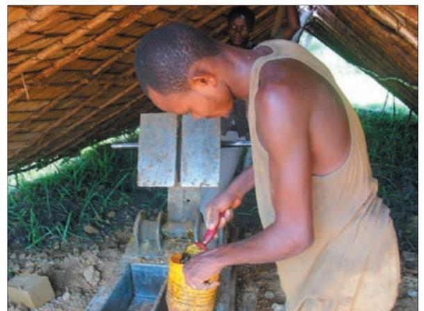
*Fabrication of the bricks - two by two*
